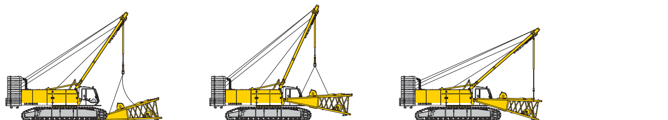
Unloading and assembly of boom foot
